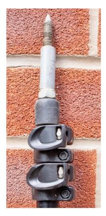
NB: The monopod is supplied with a plastic rotating clip to attached their supplied webbing strap to. I remove that strap and add my own. I also superglue the clip into position to stop it moving from the optimum position and getting in the way.
